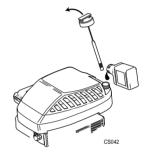
**Check oil level:** Clean around the oil filler cap before removing. With the mower on a level surface, unscrew and remove the oil filler - dipstick. Wipe oil from it with a clean cloth. Screw the oil filler - dipstick back in place, then unscrew and remove it to check the oil level.
